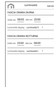
It is possible to define two time bands (day and night) and assign a different light intensity level to the display and the led for each of them. 5 brightness levels are available, plus a 0 level which corresponds to a display that is off (the led instead lights up with minimum intensity, i.e. level 1, because it can never be completely off).
